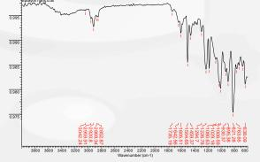
Figure 1. Non-exposed FBE FTIR spectrum
